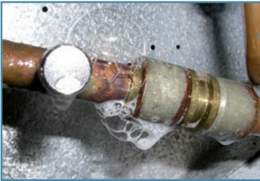
Figure 18: Bubble indicating a leak
